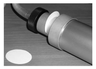
The gas sample should be drawn to the center of the combustion gas flux. The correct gas volume is sampled with 10 uniform shoots by the pump. We suggest using a retaining cone during gas sampling. Compare the darkening of the filter with the smoke index comparing table. The smoke index found should not exceed the ones defined by the current normative.
