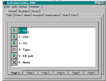
The window on the left is a parameter icon list. This list shows all possible parameters to measure (O<sub>2</sub>, CO, Tgas, Draught, etc.) and calculate measures (CO<sub>2</sub>, Efficiency, etc.). Some of these may not be available in your instrument (it depends by instrument model, installed cells, and options).
