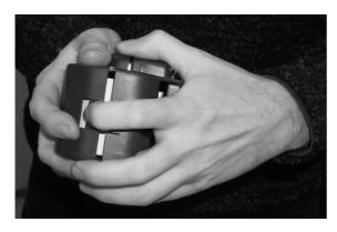
Extract the exhausted paper roll. You can use standard paper roll but you have to check before for its dimensions (max. 57mm ±1mm large).
