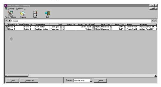
You can exclude manually one or more boilers from the list. Select or input the operator's name, connect the IR to RS232 adopter to the PC, approach the IR terminal to the analyzer IR communication windows, and press the "Send" button to send the data to the analyzer.
